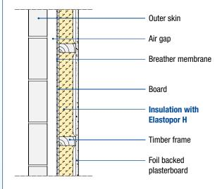
Timber frame construction with thermal insulation between studwork and ventilated outer skin (horizontal section)
