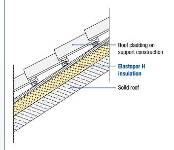
Solid pitched roof with external thermal insulation
