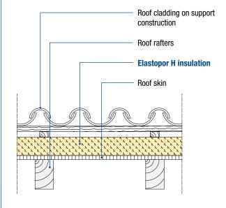
Rafter roof with visible rafters,top roof skin and external thermal insulation
