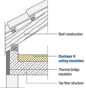
Insulation to the floor of an unheated loft/attic space
