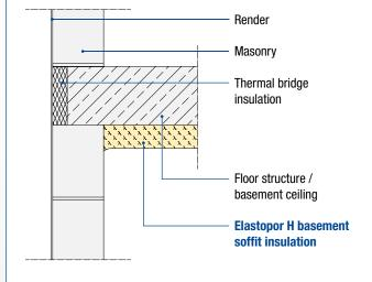
Soffit insulation for unheated basements
