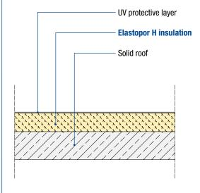
flat roof with external thermal insulation and UV protective layer
