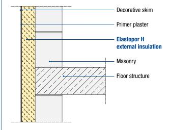
Masonry with external insulation and skim
