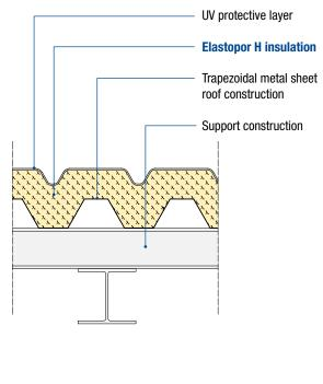
Trapezoidal metal sheet roof with external insulation and UV protective layer
