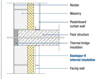
External wall with internal insulation and a lightweight or solid facing wall
