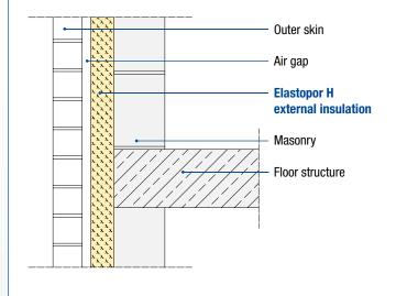
Double skin masonry with core insulation and air gap
