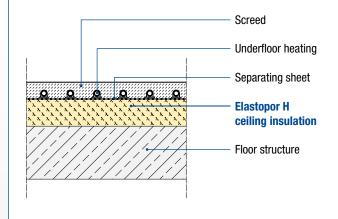
Insulation under the heating screed
