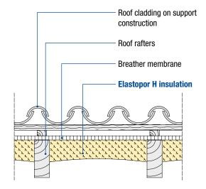
Rafter roof with membrane and internal between-rafter insulation
