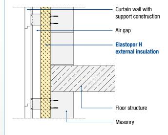
External wall with thermal insulation and curtain ventilated cladding
